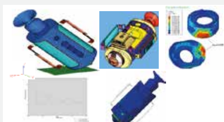
Thermal imaging camera - Drop/impact test
