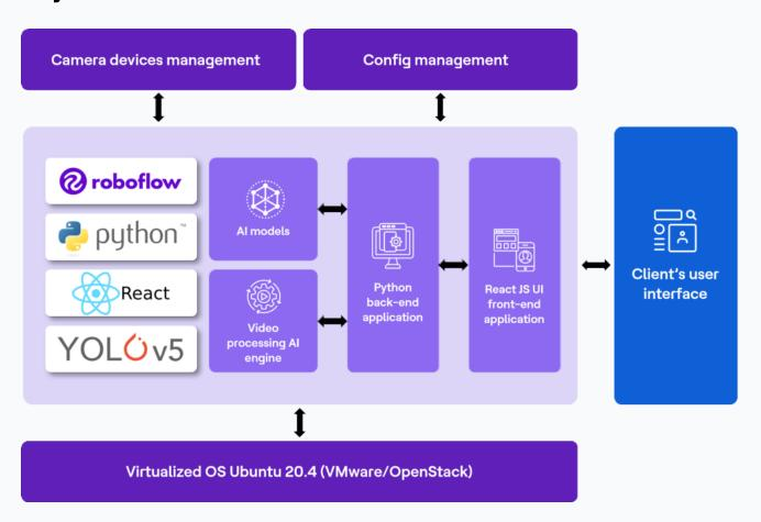
The HCLTech Smart Video Analytics solution is equipped with a robust video processing AI engine that processes live video streams. The AI model, developed using Roboflow, caters to various use cases. The platform's back-end is built in Python, while the front-end UI is powered by React JS. This highly scalable solution can be customized for specific industry verticals by developing AI models. It can be deployed both on-prem and in public cloud environments, providing flexibility to users.
