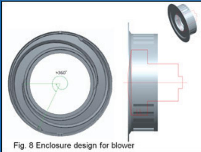
Fig. 8 Enclosure design for blower
