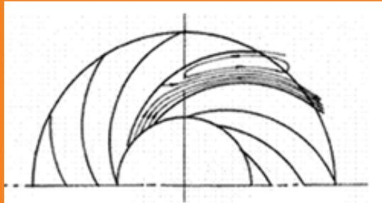
Fig. 6 Sector of the centrifugal blower, with flow separation.
