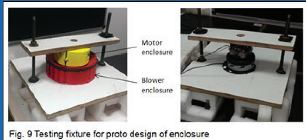
Fig. 9 Testing fixture for proto design of enclosure
