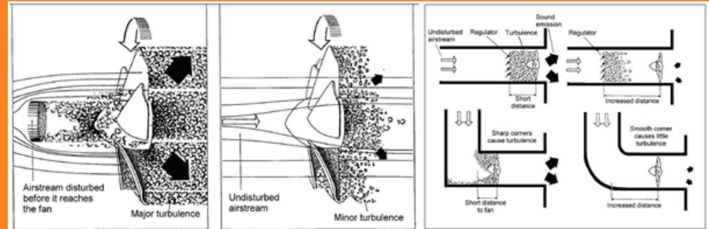
Fig. 7 Effect of initial flow condition on impeller turbulence
