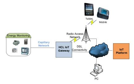
Some of the challenges/issues mentioned in the previous section can be overcome by deploying the Internet of Things (IoT) framework as shown in the figure above. Detailed scenarios/use cases leveraging IoTF are listed below:
