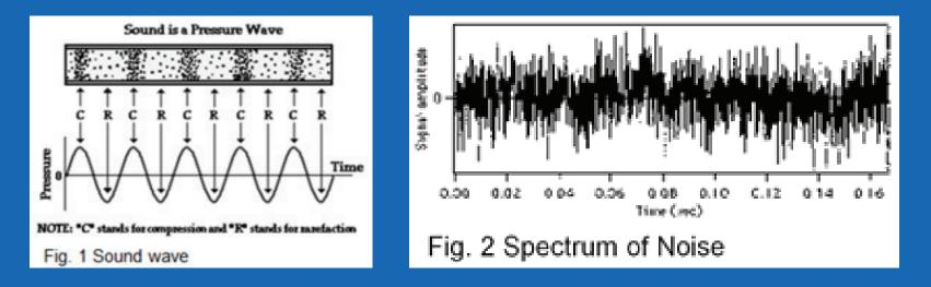
We hear different sounds from different vibrating objects because of variations in sound wave frequency and amplitude. The sensation of a frequency is commonly referred to as the pitch of a sound. The level of air pressure in each fluctuation - the wave's amplitude, determines how loud the sound is.
