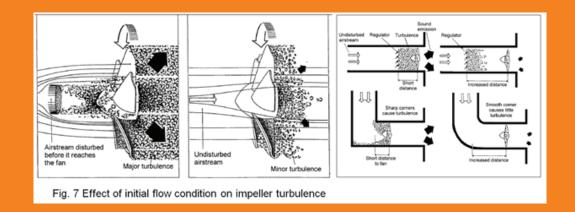
Any disturbance in the upstream of the flow has a fast exponential growth as they travel downstream, as shown in figure 7. So any small fluctuations present at the orifice, may have a large positive growth rate and quickly become very big; this was the reason that a small sealing gap near the blower orifice created a huge noise.
