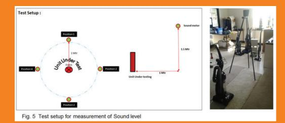
After ranking the measured values of the sound levels, two primary sources of noise were identified. The first primary source of noise is due to the mechanical vibration of the motor blower assembly, and the second is noise generated by the air blower and air exiting out of it.
