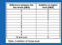
The doubling of power is represented approximately by 3dB, and a doubling of amplitude by 6dB. In Table 2 - referring to noise level addition, during a test measurement, the background noise level should always be kept 10 dB below the noise level to be measured.
